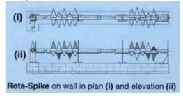
A range of support brackets are available including corner brackets, etc. Ideal for use with standard palisade fencing, etc. Rota Spike converts the perimeter into a formidable barrier against unauthorised access.
